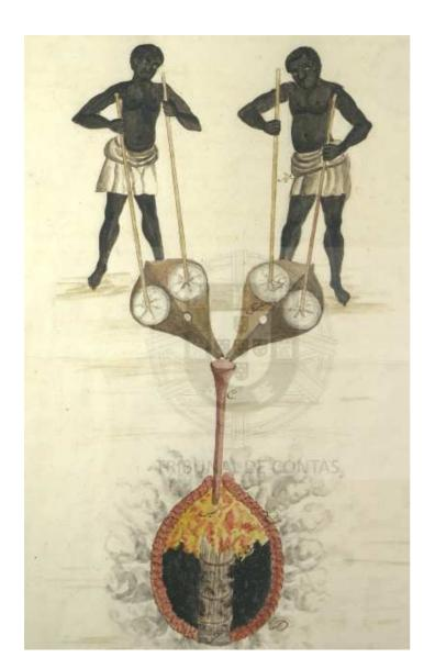
"A= This is the straw beam or 'mubu' (sic) that is placed in the middle of the furnace.
